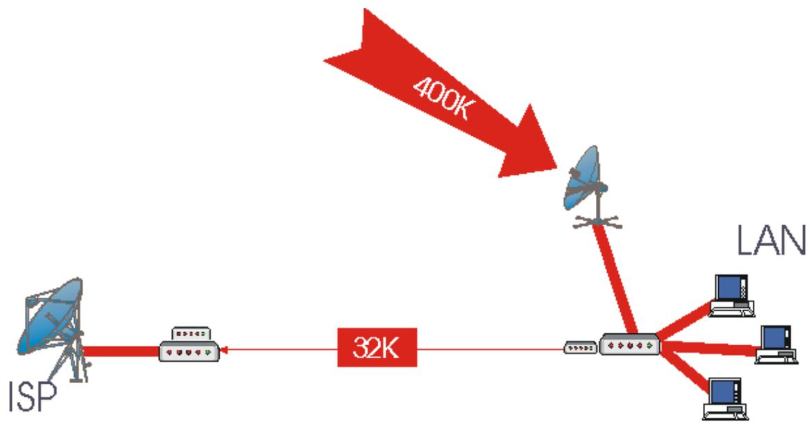
This option involves the use of a low cost receive only satellite system on one hand and a connection to an ISP via a modem connection. In this case the internet user can increase the amount of his incoming bandwidth via the VSAT and still have some means ( a 32K link) for outgoing signals.
