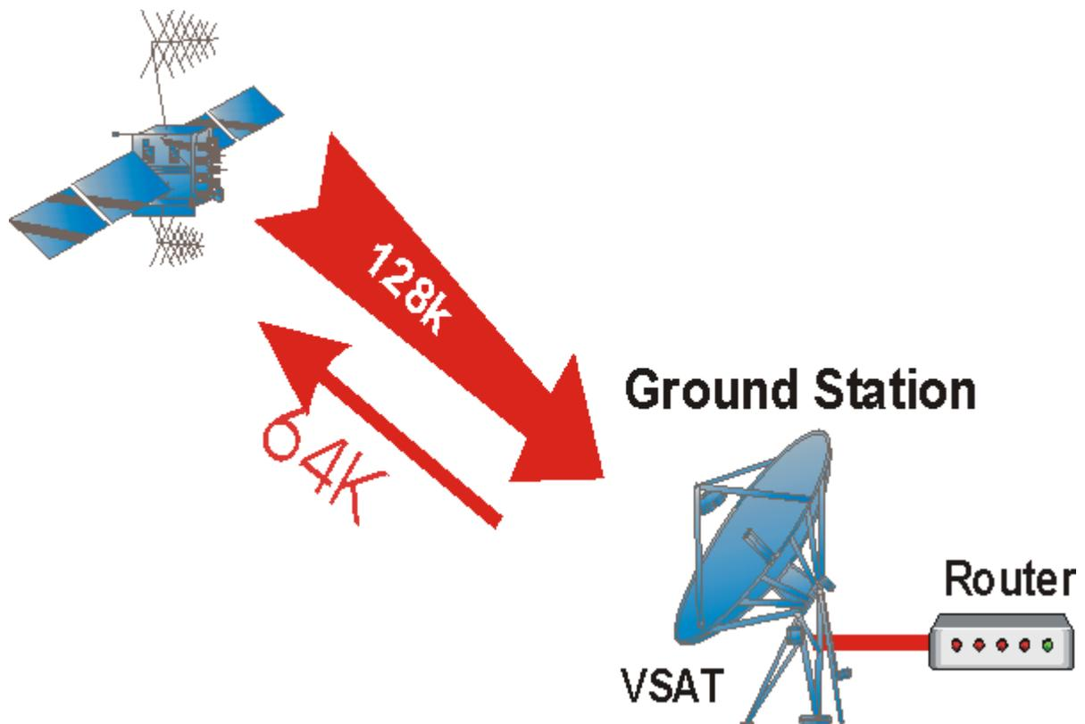
This consists of a ground station and a router and some space on a hub connected to the internet back bone.
