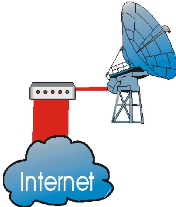
Today information is normally sent as digital signals from a ground station to a satellite. At the satellite, the signals are received, amplified, and as a rule converted into another frequency before they are sent back to another ground station. The transmission of the signals takes place by means of parabolic aerials and microwaves with wavelengths from 1 - 20 cm.
